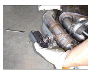
1) Using a 10mm wrench, remove the three bolts securing the exhaust actuators to the factory muffler assembly. Place them onto the mounts on the new Flowmaster units and fasten using the three bolts, tighten securely.
