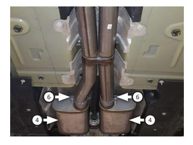
12. Place a clamp (6) onto right (2) and left (3) tailpipe then connect them to mufflers. Insert wire hangers into rubber isolators then adjust tailpipes so tips are level and centered in bumper cut-out. Tighten clamps just enough to allow for adjustment.
