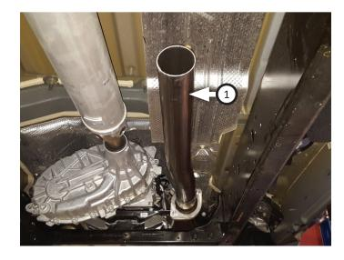
10. Fasten inlet using (x2 ea.) bolts (11), flat washers (13), lock washers (14) and nuts (12).
