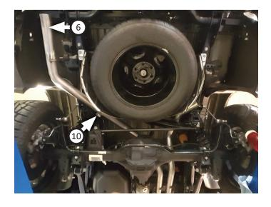
15. Place clamp (10) onto right exit pipe (7) then connect it to right overaxle pipe. Insert wire hanger into isolator then tighten clamp just enough to allow for adjustment.
