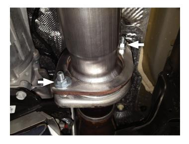
11. Place clamp (9) onto extension pipe (2) then connect them to inlet pipe. Insert wire hanger into isolater and plug in grounding wire (removed step 5). Tighten clamp just enough to allow for adjustment.
