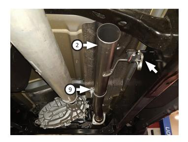
12. Place clamp (9) onto muffler (3) inlet, then connect muffler to extension. Tighten clamp on muffler inlet just enough to allow for adjustment. Place (x2) clamps (10) onto muffler outlets.
