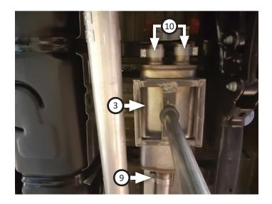
13. Route **right (5)** and **left (4) overaxle pipes** over axle and connect them to muffler outlets. Mount wire hangers into isolators then tighten clamps (x2) enough to allow for adjustment.
