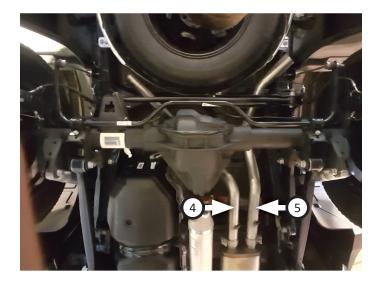
14. Place **clamp (10)** onto **left exit pipe (6)** then connect it to left overaxle pipe. Insert wire hanger into isolator then tighten clamp just enough to allow for adjustment.
