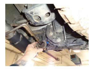
7) Remount the factory forward and rear tailpipe hangers to the frame and tighten securely. Repeat steps 6 and 7 with tailpipe **#26676M** on the left side of the vehicle.
