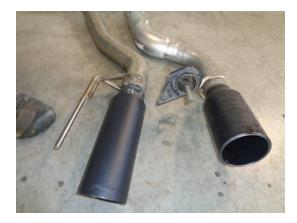
4) Place the new Flowmaster tailpipe assemblies next to the corresponding factory tailpipe. Swap both the front and rear hangers from the factory tailpipes to the new tailpipes.
