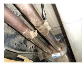
4) Support the muffler with a stand and loosen the clamp on each of the two front inlet pipes using a 15mm socket wrench. Then slide the muffler toward the rear of the vehicle to disconnect the inlet pipes and hangers from the rubber mounts on the vehicle. Lower from the vehicle and set aside.
