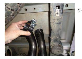
Place the provided 3" clamps onto the muffler outlets.
