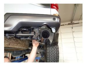
8) Place the ST462B tips onto the end of the tailpipes and adjust to the desired position. Tighten the pinch bolt on the tips enough to hold in position. Check to see that the tip is centered in the bumper cut-out and that there is clearance to the trailer hitch.
