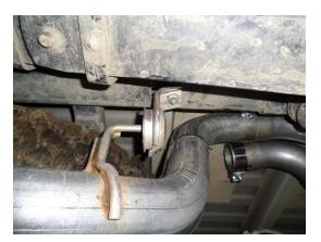
2) Loosen the two clamps connecting the tailpipes to the muffler at the over-axle slip-fit connections. Then unbolt the forward hanger mount on each tailpipe from the frame. Leave the hanger mounts connected to the tailpipes.
