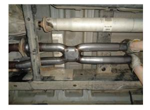
1) Place the new Flowmaster X-Pipe **#26678M** up into position behind the factory front pipes, slide the right side slip connection into the clamp and continue until the flared left connections come together. Using the included 3/8" bolts, nuts and washers, secure the two flanges together. Leave both connections slightly loose for later adjustment if needed.
