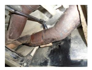
5) Support the resonator with a stand and loosen the clamp on the right inlet pipe and the two flange bolts on the left inlet pipe using a 15mm socket wrench. Then slide the resonator toward the rear of the vehicle to disconnect the inlet pipes. Lower from the vehicle and set aside.
