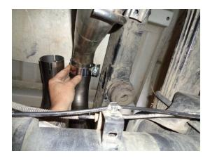
6) Place the right tailpipe **#26677M** into position over the rear axle and into the right muffler outlet.
