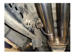
3) Place the inlet pipes of the new FlowFX muffler **#7430404-461**, into the back of the X-pipe and connect the hangers on the muffler to the rubber mounts on the vehicle. Be sure the muffler is full forward and seated. Support the muffler with a stand and tighten both clamps enough to hold but still allow for adjustment.
