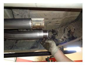
2) Place the factory band clamp from the rear of the resonator onto the left X-Pipe outlet as shown. Place the supplied  $2\frac{3}{4}$ " clamp onto the right outlet as shown.
