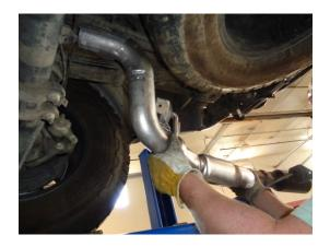
3) Unbolt the rear hanger mount on each tailpipe from the frame, leave the hangers connected to the tailpipes. Carefully slide the tailpipes toward the rear to remove from the muffler. Lower from the vehicle and set aside.
