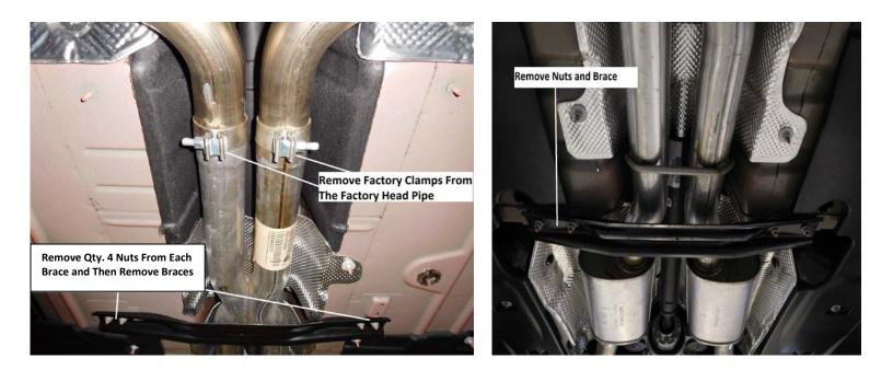
3) Place a stand under the rear of each tailpipe to support the rear of the system. Just forward of the rear differential, you will find two exhaust valve actuators, one mounted to the side of each tailpipe. Carefully unplug the wire from the actuator and tuck away for reconnection later.
