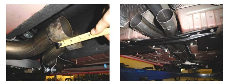
2) Place a supplied 3" clamp onto the inlet neck of both mufflers. Slide the mufflers onto the back of the Scavenger pipe assembly about 1-3/4" and support with stands. Level the mufflers and tighten the clamps enough to hold, but still allow for adjustment.
