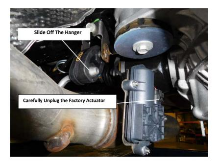
4) Slide the two hangers on each tailpipe out of the rubber mounts on the vehicle and unclip the grounding strap from the rear hanger on the right side of the vehicle. The stock system will come out as one large unit. Carefully lower the stands at the rear of the vehicle and with the help of an assistant slide the system back off of the head pipes and lower the system from the vehicle.
