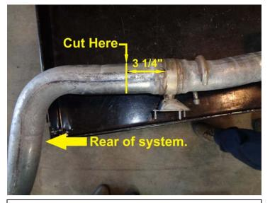
On the drivers' side of the system, Measure back 3 <sup>1</sup>/<sub>4</sub>" from the cast body of the exhaust valve and make a mark. Using a hacksaw or sawsall, cut the pipe through on this mark. After cutting, remove any burrs from the end of the pipe using a file or die grinder.
