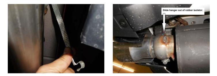
Once the factory system is out of the vehicle, turn the system over so that the hangers are to 5) the ground. Then using the measurements on the diagrams below, carefully cut the factory exhaust valves from the exhaust system, these will be re-used with the new Flowmaster system.
