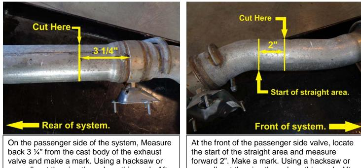
sawsall, cut the pipe through on this mark. After cutting, remove any burrs from the end of the pipe using a file or die grinder.
