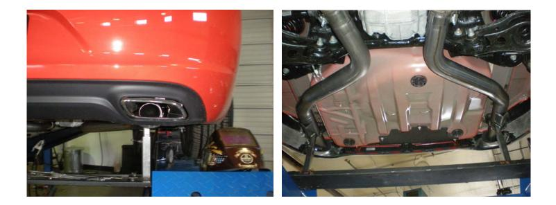
5) Reconnect the two electrical plugs removed in step 3 of the removal instructions back onto the tailpipe actuators.
