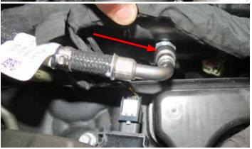
68. Remove the evap solenoid from the factory manifold. Using two (2) M6 x 25mm bolts Install the evap bracket to the supports. Install the solenoid onto the bracket using the factory rubber grommet. **NOTE: These bolts will be need to be removed later when installing the side covers.**
