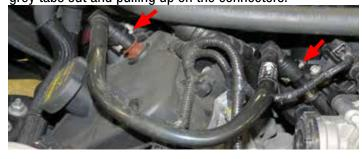
18. Disconnect the throttle body harness by pulling the red locking tab out and push down on the black tab as you pull the plug out.
