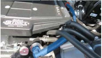
70. Using an 8mm socket, remove the throttle body from the stock manifold and install it onto the supercharger
