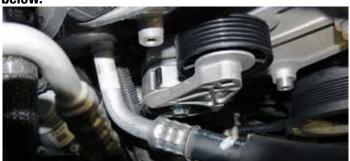
49. Install two (2) idler pulleys, one (1) 76mm and one (1) 70mm, with two (2) M8 x 20mm bolts and washers from bag #2. The smaller 70mm pulley should be installed on the uppermost boss on the tensioner bracket. Torque both idler pulley bolts to 22 ft-lbs.
