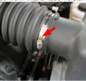
13. Remove the brake aspirator and driver side PCV hose from the back of the intake tube. Remove PCV hose from driver side valve cover and set aside. **TIP:** The brake hose is removed by pushing down the yellow clip and pulling out on connector. The PCV hose is removed by pushing out on the grey tab and pulling the connector out.
