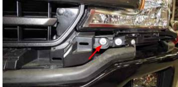
10. Pull outward on the grille tabs located in the center of the headlights. The grille should no longer be held in place by them.
