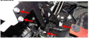
81. Install the supercharger to surge tank hose as shown using the supplied pinch clamps in bag #3.
