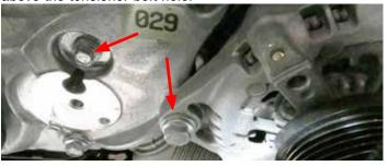
47. Using the bolts supplied in Bag #2, secure the small idler bracket by installing the M10 x 110mm bolt through the ear of the alternator, the M8 x 90mm bolt into the top front cover hole and the M10 x 45mm bolt through the center hole that was used to secure the stock tensioner. Torque M10 x 110mm bolt to 32 ft/lbs and the other two bolts to 22 ft-lb.
