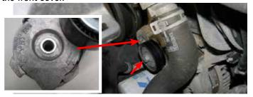
30. Using a 3/8" breaker bar or equivalent, release the tension from the secondary A/C drive tensioner and remove the A/C drive belt and discard.
