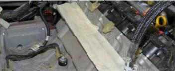
27. Remove the IMRC Solenoid from the manifold. Reconnect to the harness and zip tie out of the way. The solenoid will not be used but MUST be plugged in for
