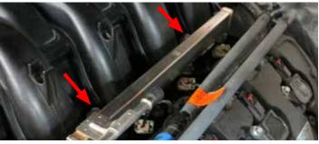
24. Using an 8mm socket, loosen the remaining six (6) intake manifold bolts. Note: Bolts can not be removed from manifold. Loosen enough so threads are disengaged from the cylinder head.
