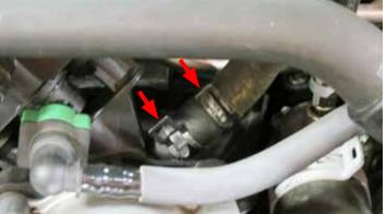
16. Disconnect the evap line from the solenoid by squeezing the green clip together at the bottom and lifting the tab up. Disconnect evap harness by pushing down the black tab and pulling plug out.
