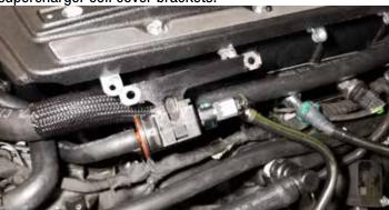
135. As a precaution, slice a 5" length of hose to wrap around the fuel line as pictured. This is to prevent the hose from rubbing on the edge of the coil cover. Secure with zip-ties.
