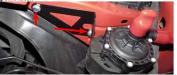
80. Remove the indicated strut tower nut and install intercooler reservoir bracket over stud. Loosely tighten the strut tower nut. Using the supplied M8 x 20mm bolt, washers and nut located in bag #3, fasten the bracket to the hole on the back of the control arm mount. Install intercooler overflow tank on bracket using the supplied M6 x 10mm bolts and align bracket so tank is sitting upright. Tighten all hardware. Do not overtighten bolts securing tank to bracket.
