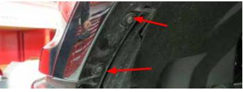
7. Pull on fender flare until the indicated clips disengage from the flare.
