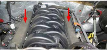
20. With the vehicle **COMPLETELY** cooled. Put rags under the fuel rail fitting and remove the fuel line from the rail. Cap off the fuel rail and fuel line with appropriate cap and plug to prevent spillage. Clean up any spilt fuel before proceeding.
