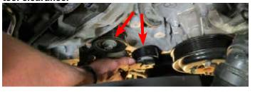
32. Remove the auxiliary water pump from the rubber
