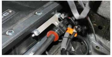
C) Connect the relay harness to the previously installed intercooler water pump and fasten the ground strap to the
