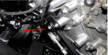
33. Remove the auxiliary water pump bracket from the front of the engine by removing the two (2) bolts and one nut securing it. The second bolt (not shown) is located further
