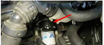
51. Using hose clamp pliers, remove factory coolant bleed hose and discard. Use the factory clamps to install the included hose show below.
