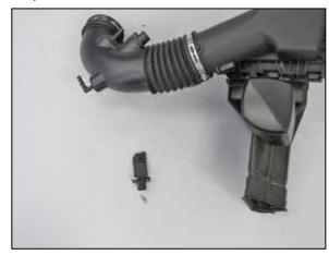
18. Remove the mass air sensor from the factory air filter housing.
