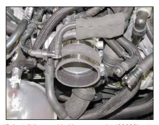
17. Install the provided hump coupler (08699) onto the throttle body and secure with the provided hose clamp.
