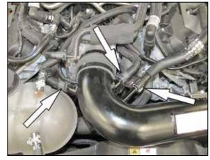
21. Connect the crank case vent, EVAP vent and idle by pass lines to the quick disconnect fittings installed into the K&N® intake tube.
