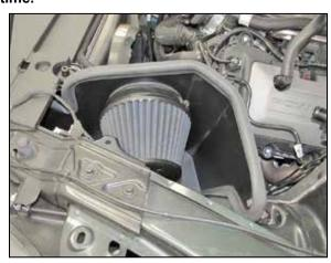
15. Install the K&N<sup>®</sup> air filter onto the adapter and secure with the provided hose clamp, then secure the heat shield and brackets to the air filter housing mounting location using the provided hardware.
