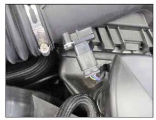
7. Release the locking tab and then disconnect the mass air sensor electrical connection.
