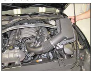
9. Loosen the hose clamp securing the intake tube to the throttle body and then remove the air filter assembly and intake tube from the engine compartment.
