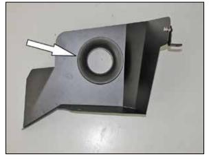
12. Install the provided filter adapter into the heat shield as shown and secure with the provided hardware.
